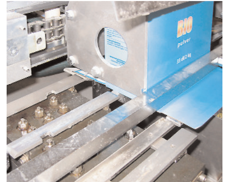
Minimal contamination on base glueing
